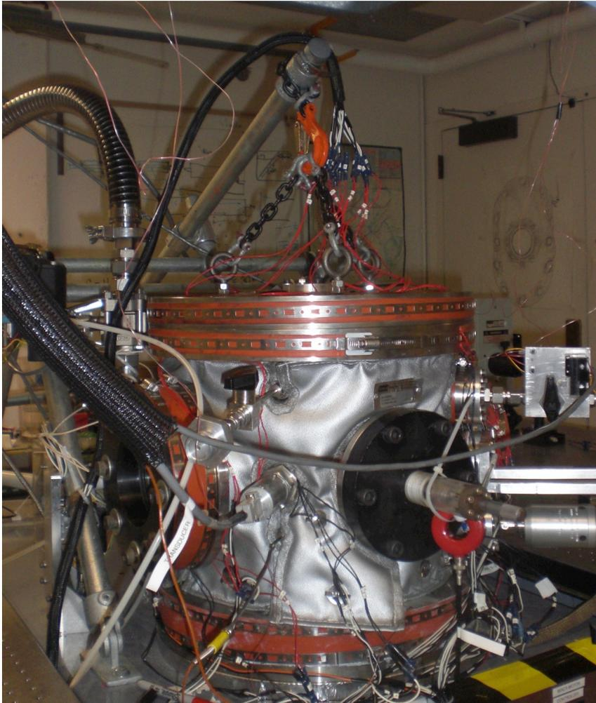
22 L, stainless steel, cylindrical combustion vessel
