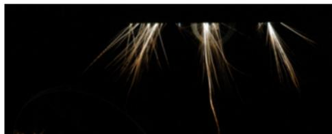
Ignition at edge of carbon fiber composite structure, Boeing
