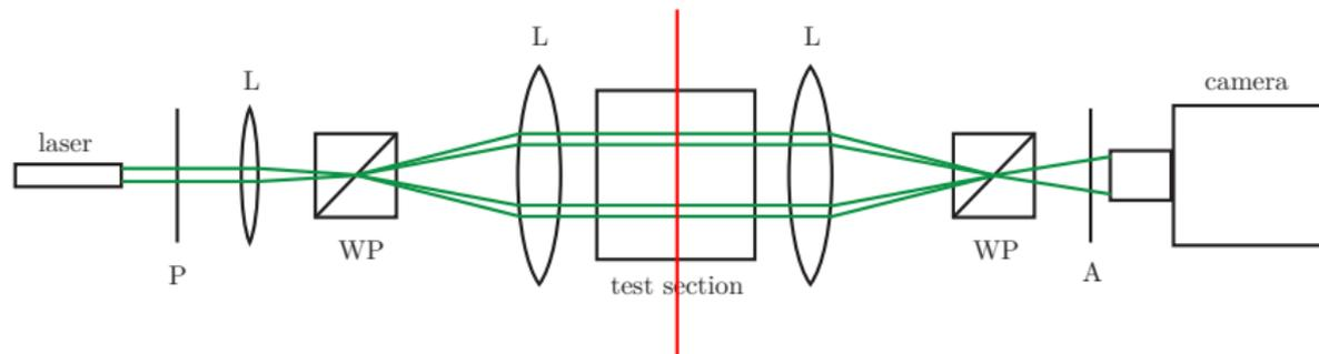
P: polarizer, L: lens, WP: Wollaston prism, A: Analyzer
