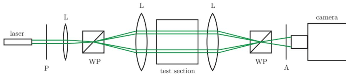
P: polarizer, L: lens, WP: Wollaston prism, A: Analyzer
